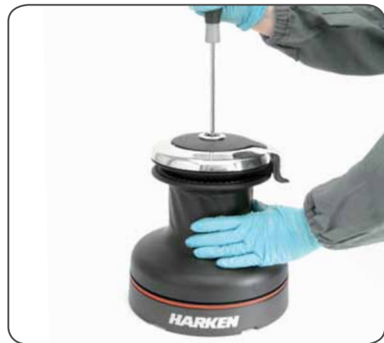
2. Unscrew the central screw ( \approx 2\text{Nm}/18\text{ in-lb} )
