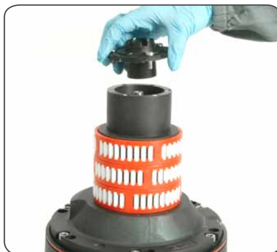
8. Remove the stripper arm housing n°21
