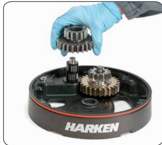
14. Remove the idler and pinion n°14
