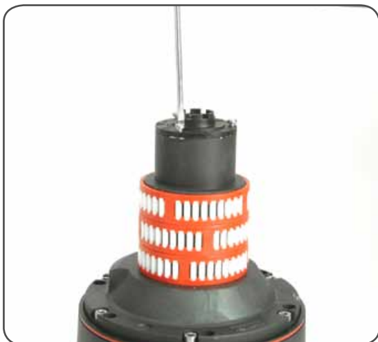
7. Completely unscrew the three screws n° 28
