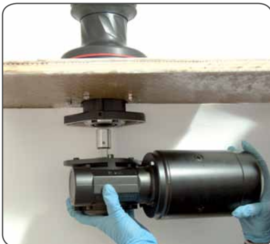
3. Position the reduction gear and motor
