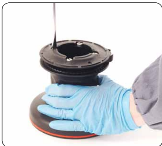
I. Unscrew the 4 screws n°26 ( \text{4Nm/35 in-lb} )
