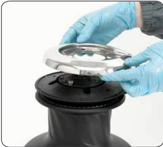
5. Remove the self-tailing arm n°27 by rotating and lifting it.
